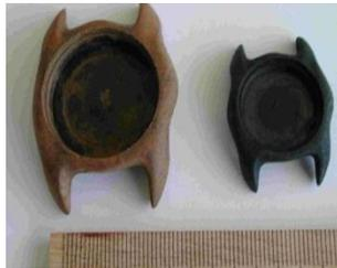
Injection moulding of ARBOFORM® with subsequent pyrolyzation results to pure carbon parts (99,9% concentration) with interesting electric conductivity properties and high dimensional stability under heat.
