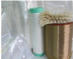
Special ARBOBLEND® grades can be processed by melt spinning to filaments with different titers.
