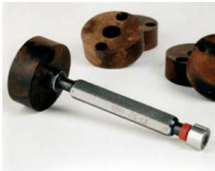
Low shrinkage qualifies ARBOFORM® for very precise items where tight tolerances are required. Injection moulded 12 H7 fit (toleranz 0,018 mm)
